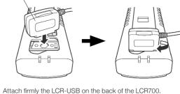
Connect the USB plug of the communication unit to your PC, then press the PC button to make it possible to communicate. [PC] will be shown on the display.
