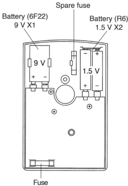
Fuse of the specified rating and type(Parts No. F1176)
