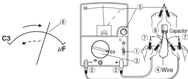
The pointer moves to right direction scale by the charge current to the capacitor. However, the pointer starts gradual returning from a certain point. Read the indicated maximum value on C3 scale.
