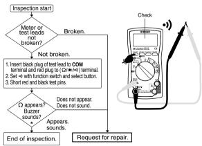
\* If nothing appears on the display, the batteries might have been discharged completely.
