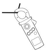
Clamp and pull the wire by trans core(CT)
