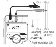
ACV and DCV are automatically detected
