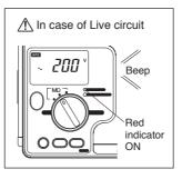
NIf the object to be measured is a live circuit (≥30 V AC/DC), the voltage is displayed, buzzer sounds, and the ALARM indicator lights up. In this case, the test voltage cannot be output by pressing the MEASURE or LOCK button. Disconnect the power supply from the object to be measured and try again.
