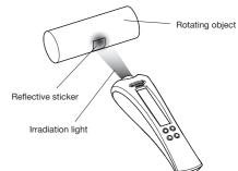
1) Turn the instrument ON and set the desired measurement mode Each press of the MODE button switches the measurement mode in the following cycle:
