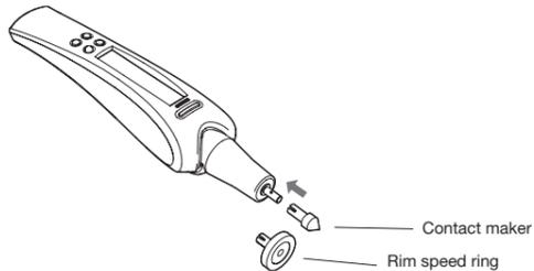
\* Select the rim speed ring when measuring the velocity of a belt conveyor or similar object (Travel distance per minute in m/min or travel distance per second in m/s).
